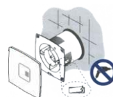
Brzim zatezanjem žabica u bilo koji otvor Fast installation by tightening hooks into any opening
